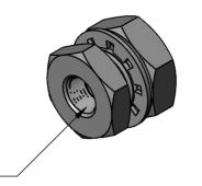
1/8 NPT PIPE SIZE, 27 THREADS PER INCH, 0.26" THREAD ENGAGEMENT—
