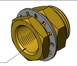
3/4 NPT PIPE SIZE, 14 THREADS PER INCH, 0.55" THREAD ENGAGEMENT—
