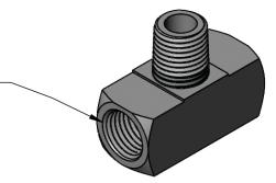
1/4 NPT PIPE SIZE, 18 THREADS PER INCH, 0.40" THREAD ENGAGEMENT—
