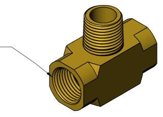
1/2 NPT PIPE SIZE, 14 THREADS PER INCH, 0.53" THREAD ENGAGEMENT—
