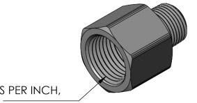
1/2 NPT PIPE SIZE, 14 THREADS PER INCH, 0.53" THREAD ENGAGEMENT
