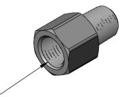
1/4 NPT PIPE SIZE, 18 THREADS PER INCH, 0.40" THREAD ENGAGEMENT -
