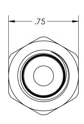
1.06 .70 .83 - 1/8 NPT PIPE SIZE, 27 THREADS PER INCH, 0.26" THREAD ENGAGEMENT
