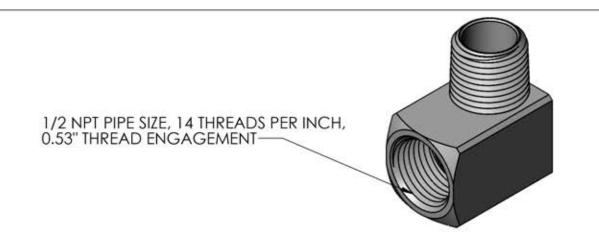
1/2 NPT PIPE SIZE, 14 THREADS PER INCH, 0.53" THREAD ENGAGEMENT—
