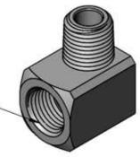
1/8 NPT PIPE SIZE, 27 THREADS PER INCH, 0.26" THREAD ENGAGEMENT—
