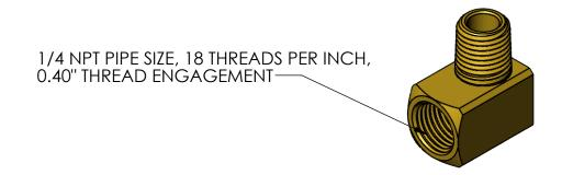
1/4 NPT PIPE SIZE, 18 THREADS PER INCH, 0.40" THREAD ENGAGEMENT—
