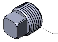
3/8 NPT PIPE SIZE, 18 THREADS PER INCH, .41" THREAD ENGAGEMENT
