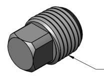
\_1/4 NPT PIPE SIZE, 18 THREADS PER INCH, 0.40" THREAD ENGAGEMENT
