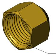
\_1/2 NPT PIPE SIZE, 14 THREADS PER INCH, 0.51" THREAD ENGAGEMENT
