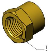
\_ 1/8 NPT PIPE SIZE, 27 THREADS PER INCH, 0.30" THREAD ENGAGEMENT
