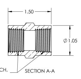
1/2 NPT PIPE SIZE, 14 THREADS PER INCH, \_ 0.55" THREAD ENGAGEMENT
