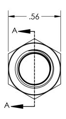
1/8 NPT PIPE SIZE, 27 THREADS PER INCH, 0.34" THREAD ENGAGEMENT
