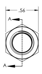
1/8 NPT PIPE SIZE, 27 THREADS PER INCH, 0.34" THREAD ENGAGEMENT
