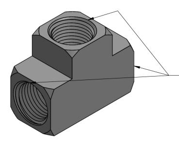
3/8 NPT PIPE SIZE, 18 THREADS PER INCH, 0.47" THREAD ENGAGEMENT
