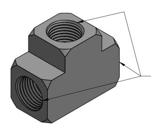
1/8 NPT PIPE SIZE, 27 THREADS PER INCH, 0.26" THREAD ENGAGEMENT
